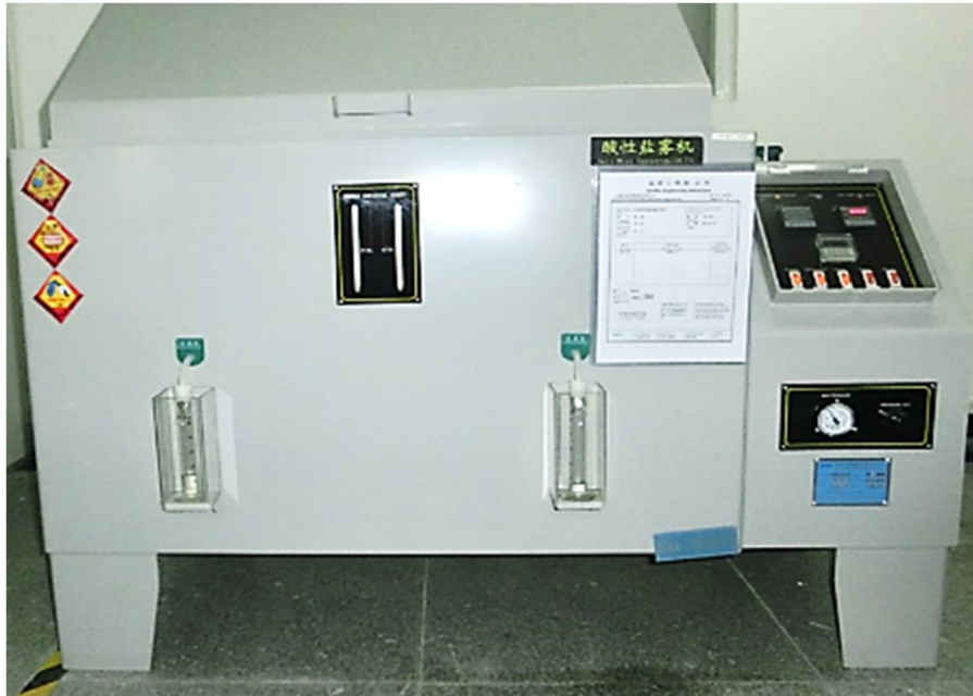
ASS: Acid Salt Spray tester
