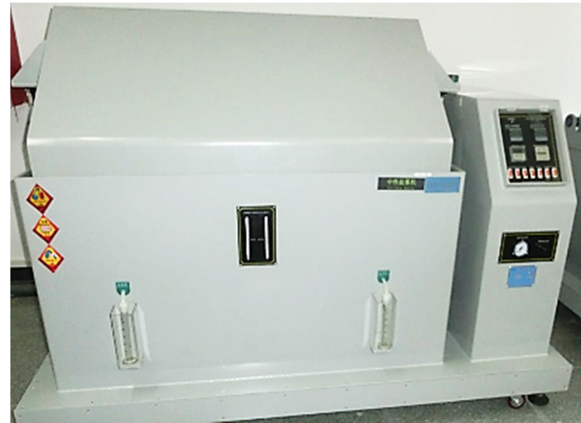
NSS: Neutral Salt Spray tester
